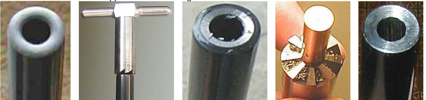
Left to Right - factory barrel, ready to start, after a few turns, remove shavings, ready to finish
